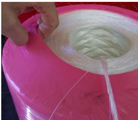
Do not pull out the strand which comes out of the wrap (which is tied with the strand coming out of the inside of the bobbin). Just cut it.
